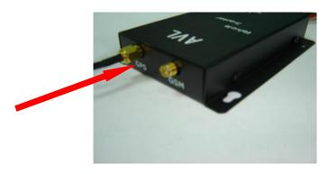
GPS antenna is used to receive satellite signals in the sky. It should be positioned at a place where it will have an unobstructed view of the sky. The ideal location is top of the dashboard or close to the rear window of the car.
